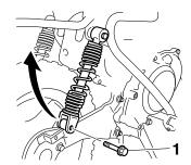
1. Rear shock absorber mounting bolt
