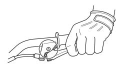
The pivoting points of the front and rear brake levers must be lubricated at the intervals specified in the periodic maintenance and lubrication chart.
