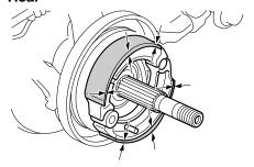
If the lining thickness of a brake shoe is less than 1.5 mm (0.06 in), have a Yamaha dealer replace the brake shoes as a set.
