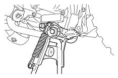
The operation of the centerstand should be checked before each ride, and the pivots and metal-to-metal contact surfaces should be lubricated if necessary.
