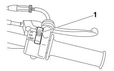
1. Engine stop switch "OFF/RUN/START"
