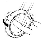
The front and rear wheel bearings must be checked at the intervals specified in the periodic maintenance and lubrication chart. If there is play in the wheel hub or if the wheel does not turn smoothly, have a Yamaha dealer check the wheel bearings.
